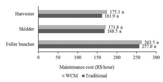
**Figure 4.** Maintenance costs per worked hour of the wood harvesting machines submitted to the traditional and the WCM mechanical maintenance models.
