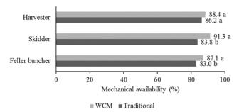
**Figure 2.** Mechanical availability of wood harvesting machines subject to the traditional and WCM mechanical maintenance models.
