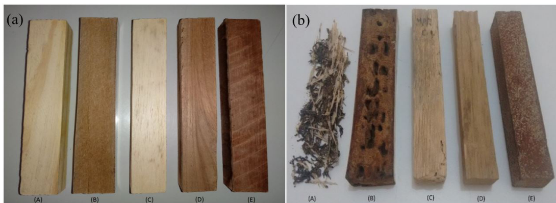
Figure 1. (a) Wooden stakes of the four forest species and of MDF prior to exposure in the soil and (b) after being attacked by Coptotermes gestroi . (A) Pinus elliottii ; (B) MDF; (C) Schefflera morototoni ; (D) Allantoma lineata ; and (E) Manilkara huberi .
