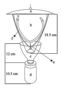
**Figure 2.** Front view: (a) covering plate; (b) interceptor panel "Semi-funnel"; (c) collector funnel; (d) collecting bottle; (e) wire fastener; (f) deposit of ethanol. Source: Carvalho & Trevisan (2015).
