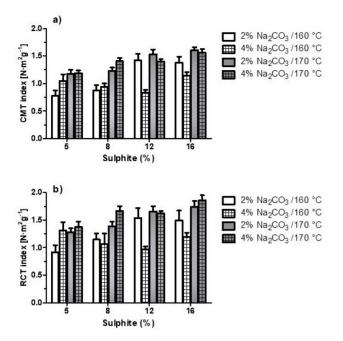
**Figure 2.** CMT (a), and RCT (b) properties of paper sheets produced from *E. globulus* bark pulps elaborated using 2% and 4% of sodium carbonate at 160°C and 170°C in different sulphite concentration.
