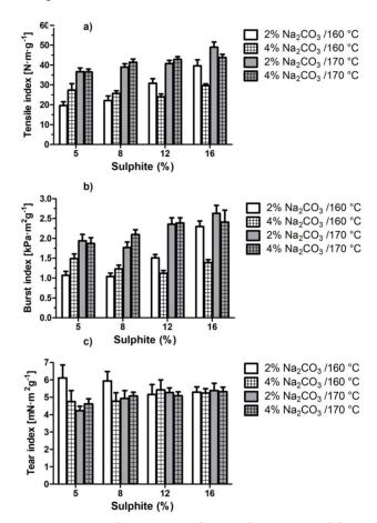
**Figure 1.** Strength properties of paper sheets prepared from *E. globulus* bark pulps using 2% and 4% of sodium carbonate at 160°C and 170°C in different sulphite concentration: (a) tensile index, (b) burst index, (c) tear index.
