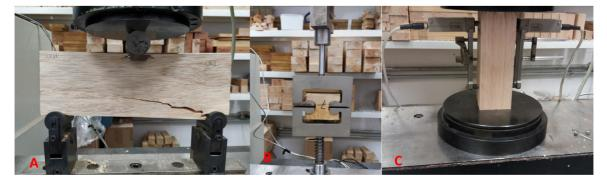
Figure 3. A – Bending test - ISO 13910 (2005); B – Tensile test - ABTN NBR 7190 (1997); C - Compression test parallel to the grain - ABTN NBR 7190 (1997).
